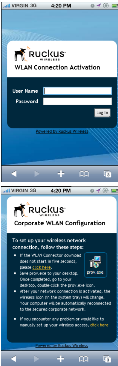
FIGURE 95 Activate device using the WLAN Connection Activation screen, and download activation file
